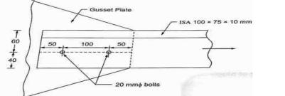
(b) Design a suitable single section to carry a factored tensile force of 210 kN assuming a single row of M20 bolts. The yield strength and ultimate strength of the material is 200 MPa and 410 MParespectively. The length f the member is 3
